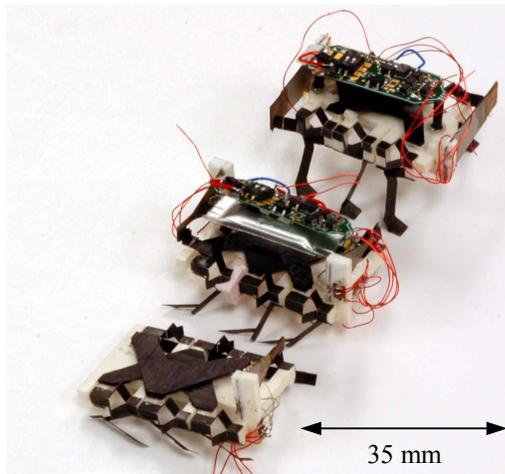
Fig. 13 Three Prototype Crawling Mechanisms
