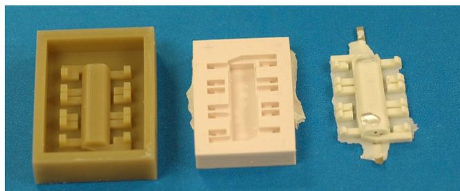
Fig. 5 Three Step Molding Process
