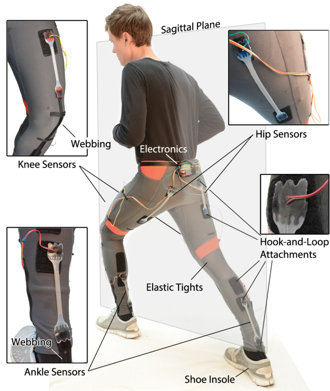
Figure 1: Soft strain sensors were placed at each lower limb joint to capture motion in the sagittal plane. In the case of the knee and ankle sensors (insets on left) webbing directed motion over the joint.
