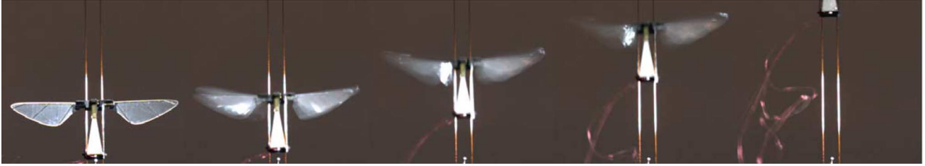
Fig. 9. First tethered flight of an at-scale robotic insect. From a video sequence spaced at approximately 100 ms intervals.
