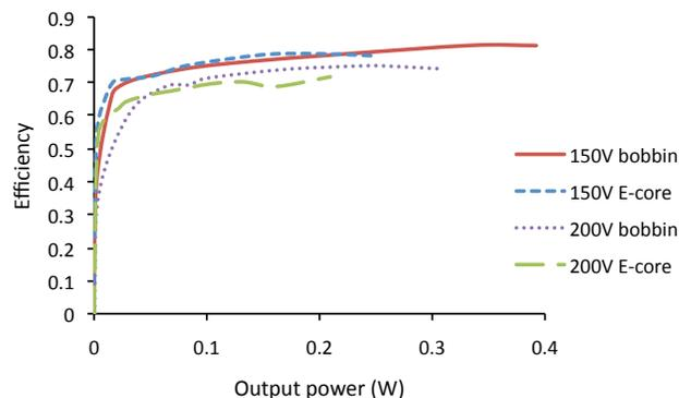
Fig. 12. Efficiency vs. output power of tapped inductor boost converters using bobbin core and laser micromachined E-core.
