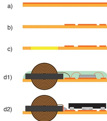
Fig. 9. Substrate fabrication and circuit assembly process: a) copper-laminated polymer substrate, b) flex circuit lithography, c) laser micromachining of through-holes, and d1) placement, bonding, and polymer encapsulation of bare-die components, or d2) placement and reflow soldering of chip-scale components.
