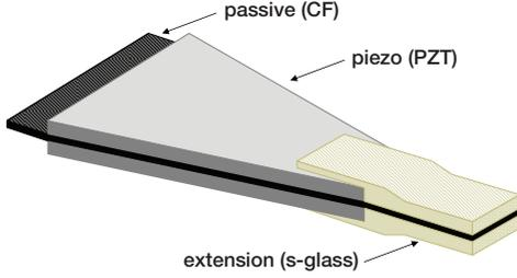
Fig. 2. Piezoelectric bimorph structure.
