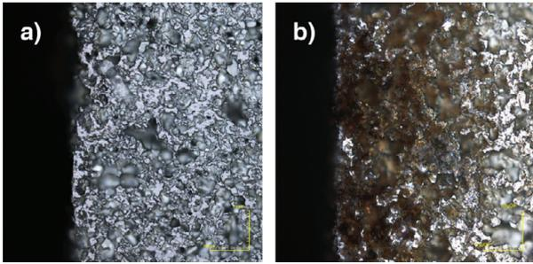
Fig. 14. Top view of ferrite edge manufactured using traditional sintering processes (a) and laser micromachining (b) under identical lighting conditions at 50X magnification (scale bars 40 $\mu$ m).
