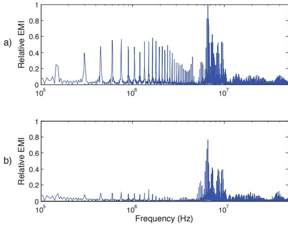
Fig. 13. Relative EMI spectra measured 1cm from bobbin core (a) and E-core (b).
