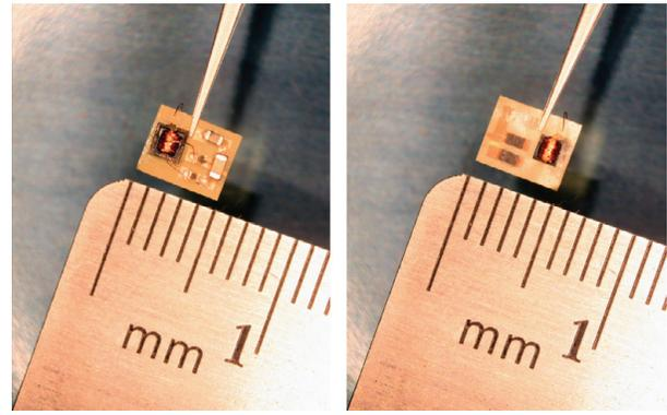
Fig. 15. Front and back view of 20mg tapped inductor boost converter.
