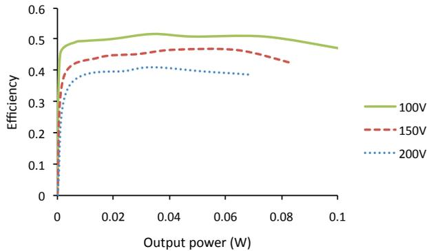
Fig. 16. Efficiency vs. output power of 20mg tapped inductor boost converter at three output voltage levels.
