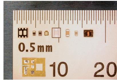
Fig. 8. Chip-scale, bare-die, and passive components used in ultra-light high-voltage power circuits. Left to right: Dual 190V nFETs, 30V nFET, 325V diode, bare-die 240V nFET (decapsulated with sulfuric acid), bare-die 60V nFET (commercially available), 0.1 $\mu$ F 200V capacitor, 4.2 $\mu$ F 6.3V capacitor, 5mg laser micromachined inductor. Bottom: Flex circuit substrate manufactured from DuPont Pyralux laminate.
