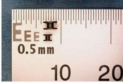
Fig. 6. E-cores fabricated by laser micromachining and bobbin cores salvaged from commercial inductors.
