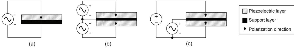
Fig. 4. Unipolar drive methods for piezoelectric actuators: unimorph (a), bimorph with alternating drive (b), and bimorph with simultaneous drive (c).
