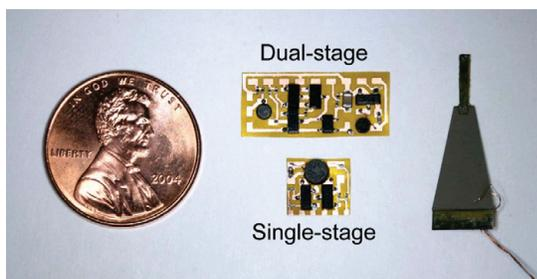
Fig. 10. Implementations of piezoelectric drive circuits next to piezoelectric bimorph actuator [5].
