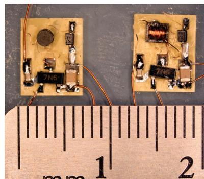
Fig. 11. Implementations of the tapped inductor boost converter using bobbin core (left) and laser micromachined core (right). All other circuit components are kept the same.
