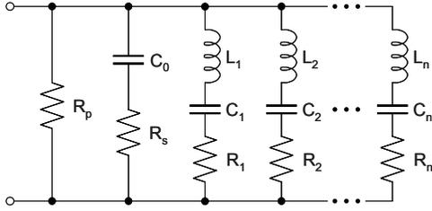
Fig. 3. Piezoelectric element equivalent circuit.
