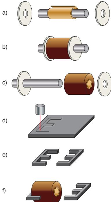
Fig. 7. Fabrication of custom magnetic components: a) temporary bobbin formation using Kapton liner and laser-cut plastic discs, b) coil winding, c) temporary bobbin removal, d) laser micromachining of ferrite core, e) core release, f) component assembly.
