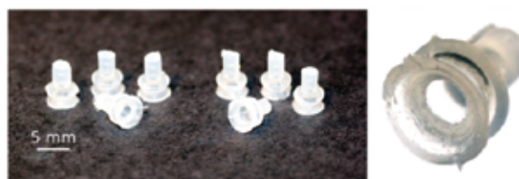
Fig. 2. Left, fabricated prototypes of suction based soft grippers, right, zoomed view of the gripper.
