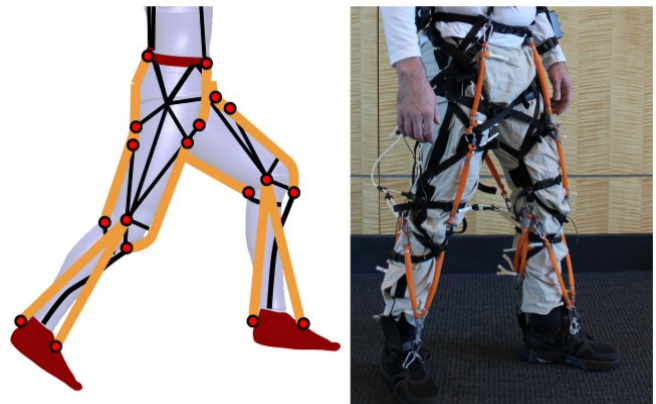
Figure 1. A lightweight, non-restrictive soft lower extremity exosuit that can provide gait assistance through pneumatic actuators (orange) that span the hip, knee and ankle joints.
